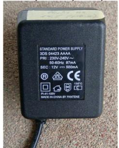
Fig.2.3 Typical 12V power supply for cordless telephones
