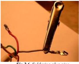
Fig.2.6 Soldering plug pins
