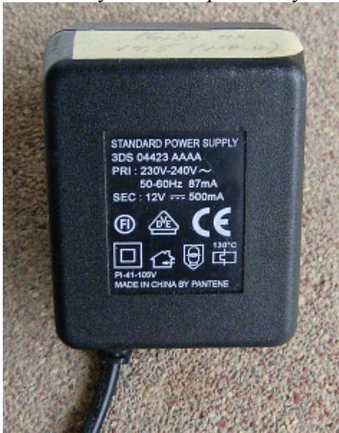
**Fig.2.3** Typical 12V power supply for cordless telephones
