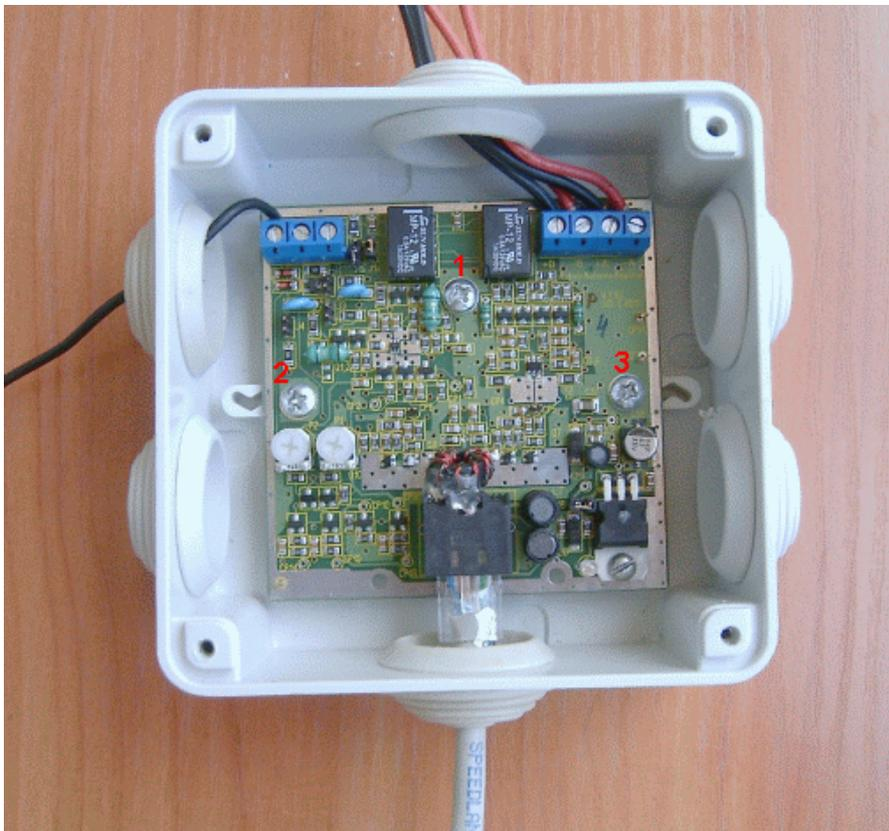
**Fig. 2.16** Mounting the amplifier board into the box
